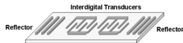
Figure 5: Schematic diagram of a SAW component
