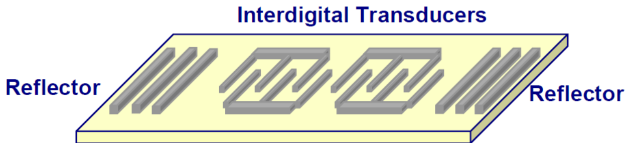
Fig.1: Simplified internal structure of a two-port SAWR
